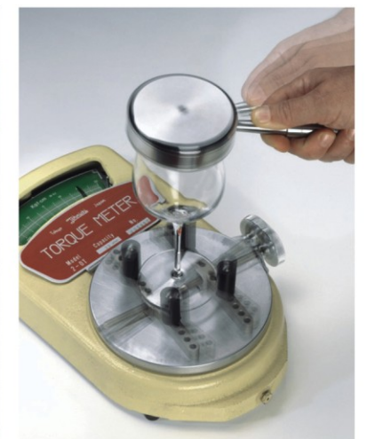
Stem twisting test 杯挺扭曲测试
